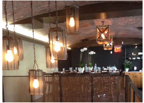
McNICHOLS® Wire Mesh, Designer Mesh, TECHNA™ 8169, Bronze, Bronze Alloy, Woven – Intercrimp Weave, 74% Open Area – various uses in a New York restaurant
